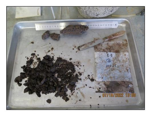
Plate 1 – Polymer Retrieved in Split Spoon Boring B-3 from 23.5 to 25-feet below grade (N=24 medium dense – previously WR)
